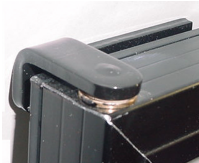
New hinge installed
